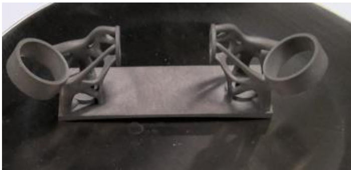
Figure 13: AM-produced LPT bracket
