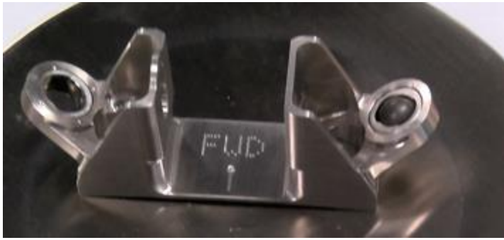
Figure 12: Traditionally manufactured LPT bracket
