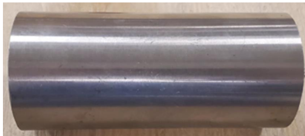
Figure 18: Inconel 718 bar stock for traditional manufacturing
