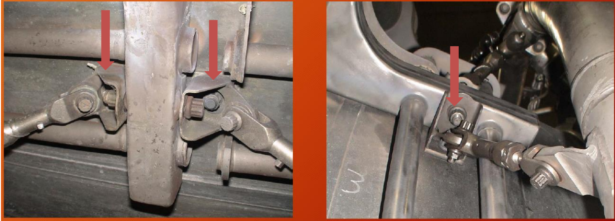
Figure 33: Installed LPT bracket
