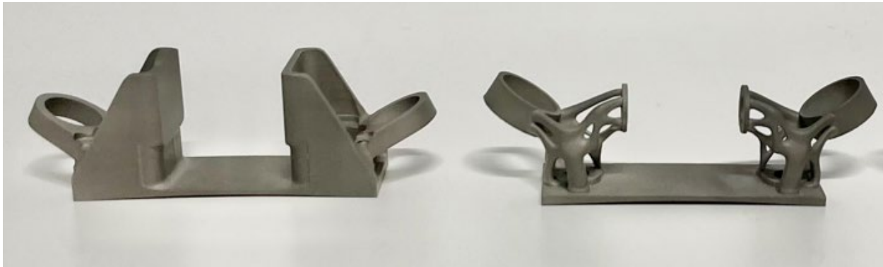
Figure 14: Side-by-side comparison of the traditional and additive LPT brackets
